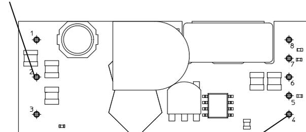
Pin 4 for measurement of minimum Solder joint temperature,  $T_{PIN}$
