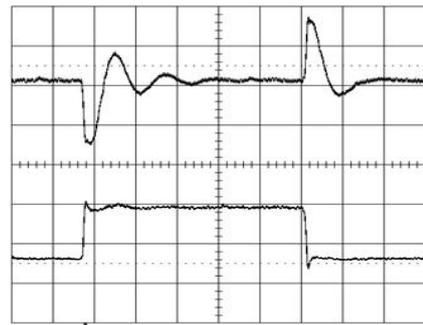
Output voltage response to load current step-change (6.25-18.75-6.25 A) at:
